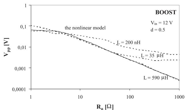
Fig. 10. The dependence of the ripples of the output voltage on the load resistance for the boost converter
