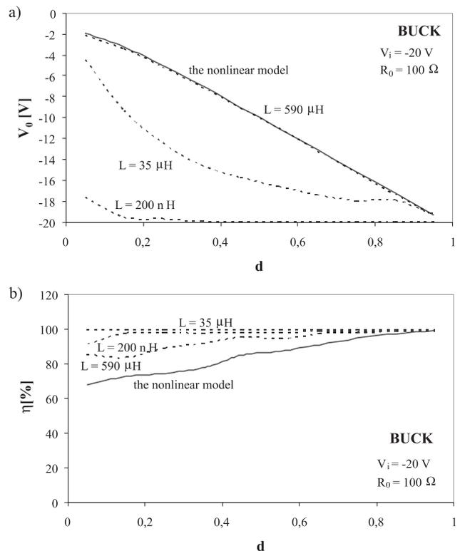
Fig. 4. The dependence of the output voltage (a), and the efficiency (b) on the duty factor for the buck converter
