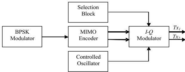
Fig. 2: Transmitter design of a MIMO system
