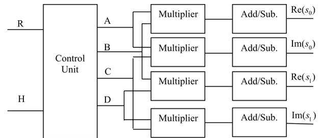
Fig. 3: Block diagram of hardware design of MIMO decoder
