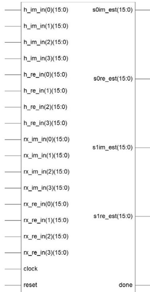
Fig. 7: Top level schematic of MIMO decoder
