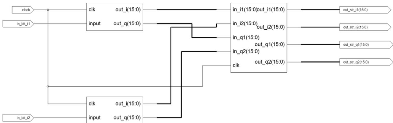
Fig. 5: Schematic of MIMO transmitter
