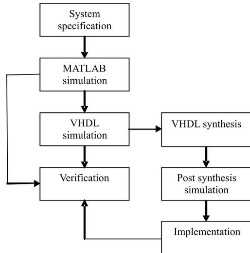
Fig. 4: Design steps of FPGA implementation
