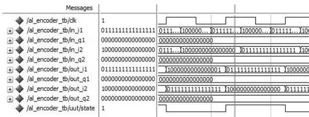
Fig. 6: Simulation result of MIMO encoder
