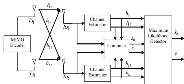
Fig. 1: Block diagram of MIMO system
