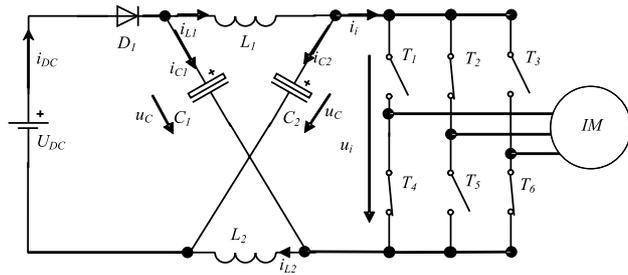
Fig. 3: Z-Source Inverter with induction motor
