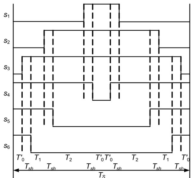
Fig. 6: Modified SVM switching pattern showing the uniform distribution of  $T_{sh}$
