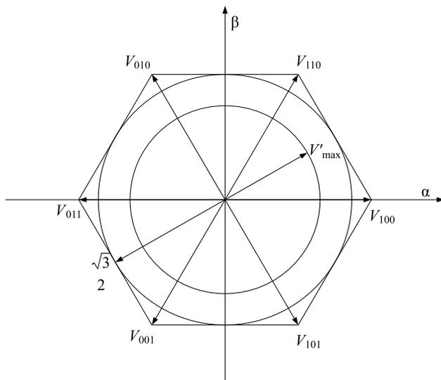
Fig. 7: Modified trajectory of the clamped voltage vector  $V'_{max}$
