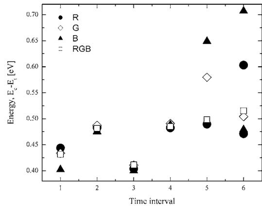
**Figure 5:** Calculated trap energy levels for PD responses to simultaneous voltage and red, green, blue and red-green-blue light pulses presented in Fig. 1, respectively. The time intervals corresponds to one in which the changes in response shapes occurs and are exponential in nature.
