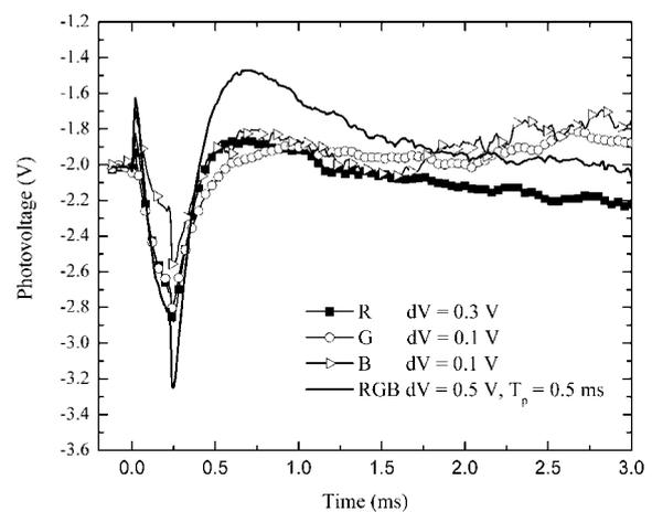
**Figure 1:** PD responses to simultaneous light and voltage pulses under the illumination of R, G, B and RGB LED. The voltage pulse amplitudes ( $dV$ ) were 0.3, 0.1, 0.1 and 0.5V, respectively. Pulse duration ( $T_p$ ) of 0.5 ms was the same in all cases.
