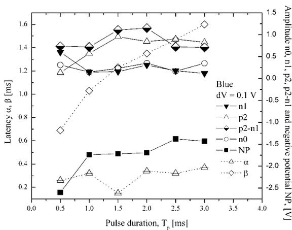
**Figure 4:** Amplitudes n0, n1, p2, p2-n1, negative potential NP, and latency  $\alpha$ ,  $\beta$  of n1 and p2 peaks of PD responses to simultaneous voltage and blue light pulses respectively as a function of pulse duration,  $T_a = 0.5 \div 3$  ms.
