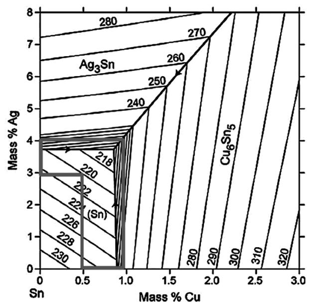
**Figure 3:** Sn-Ag-Cu ternary phase diagram (Ma and Suhling 2009).
