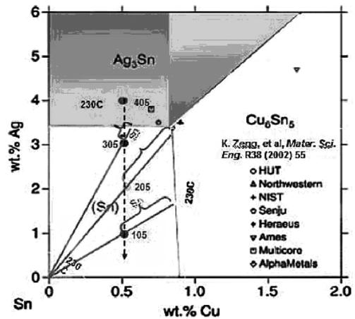
**Figure 6:** Sn-rich region of Sn-Ag-Cu ternary phase diagram. Variation of Ag content (with fixed Cu content of 0.5%) is indicated by vertical line. The tie line is also shown for representative SAC alloys (Kim, Suh et al. 2007).
