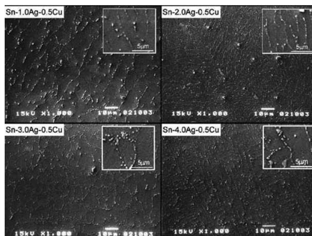
**Figure 4:** The initial microstructure of Sn-xAg-Cu bulk solders (Kariya, Hosoi et al. 2004).
