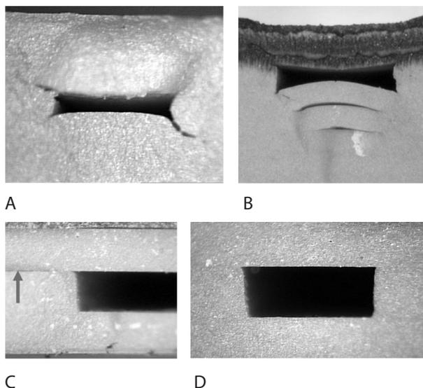
**Figure 7:** Lamination problems in fluidic structures: A) crushing of cavities; B) deformations combined with poor interlayer lamination below cavity due to absence of pressure; C) poor lamination, at arrow; D) good lamination with low deformation, with correct parameters [13].
