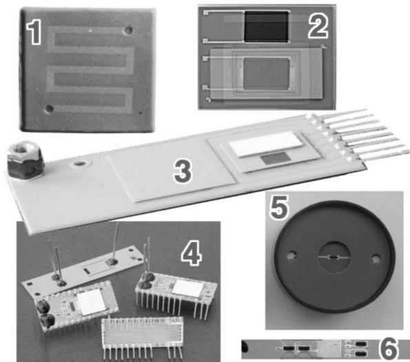
**Figure 1:** Example LTCC structures (see table 2) (1-3) Meander channel (1) and heater module (2) for gas viscosity sensor (3, with membrane) [18-20]; 4) chemical microreactor with complex fluidic circuit [16, 20]; 5) thermal bubble inclinometer (with membrane) [9]; 6) cantilever sensor for low forces [9, 16, 21, 22].
