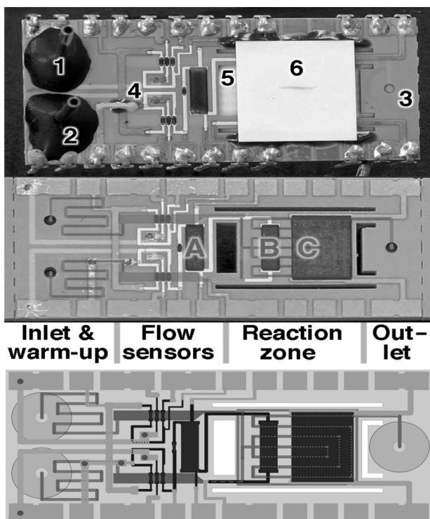
**Figure 5:** Chemical microreactor: device (top), LTCC module with superposed fluidic layout (middle) and complete electrical & fluidic layout (bottom). 1) Inlets & heat-up meanders; 2) outlet; 3) flow sensors; 4) bottom alumina heat spreader, below LTCC; 5) alumina heat shield for reaction zone. A) Thermistor for body temperature; B) thermistor for reaction zone temperature; C) resistor for heat output calibration.
