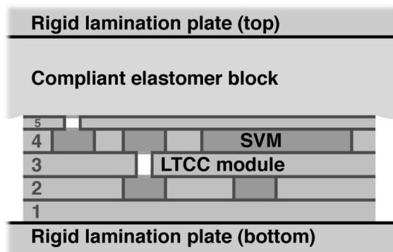
**Figure 3:** Filling crushable cavities with SVM, with pseudo-isostatic lamination (isostatic or uniaxial also possible).
