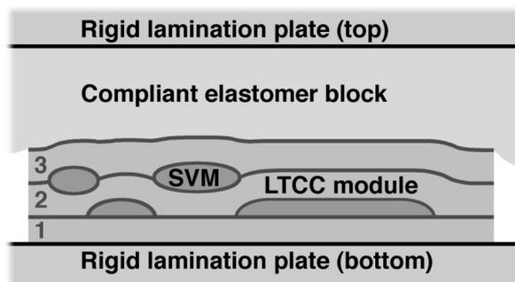
**Figure 4:** Pseudo-isostatic (similar to isostatic, where the bottom face is also deformed) lamination of LTCC modules, with printed SVM to create cavities.
