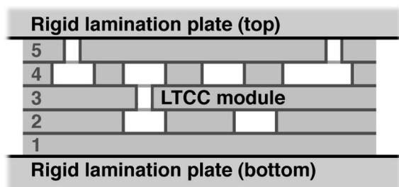
**Figure 2:** “Cut-and-laminate” structuration of LTCC: uniaxial lamination of previously processed sheets between rigid metal plates.
