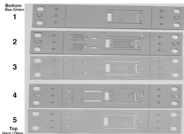
**Figure 6:** Chemical microreactor: LTCC layers, in unfired state, showing cut-outs for fluidic channels and thermal decoupling of calorimetric reaction zone. 1) Bottom wall; 2) bottom fluidic layer; 3) fluidic separation layer; 4) top fluidic layer; 5) top lid.
