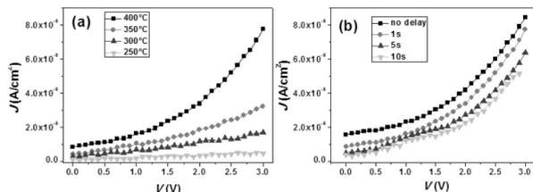
**Figure 1:** (a) Current density versus applied voltage characteristics of the 8:1:1 thin films recorded after a delay time of 1 s at each measurement point. (b) *J-V* characteristics recorded with different delay times for the 8:1:1 thin film processed at 400 °C.
