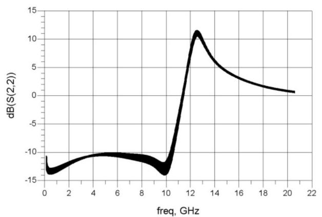
**Figure 9:** The output return loss
