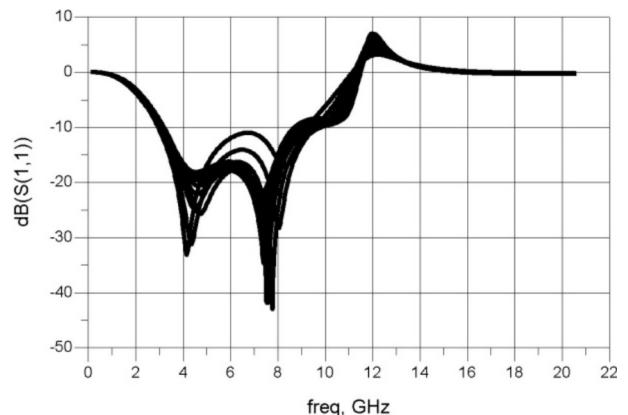
**Figure 8:** The input return loss
