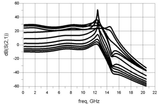
**Figure 7:** variable gain of proposed VGDA
