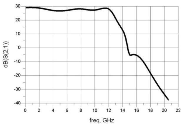
**Figure 6:** Gain ( $S_{21}$ ) of proposed VGDA
