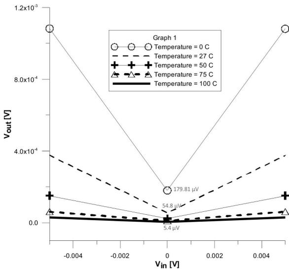
**Figure 10:** Simulated results for DC characteristics at zero crossing regions among different temperatures.
