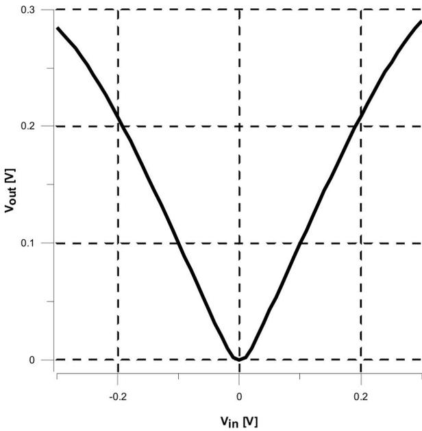
**Figure 5:** DC transfer characteristic of the proposed rectifier.
