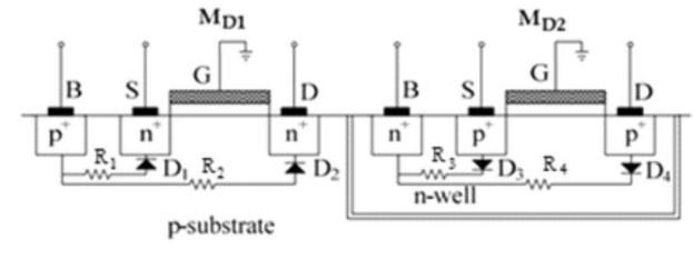
Figure 3: Cross-section of  $M_{D1}$  and  $M_{D2}$  transistors in a p-substrate CMOS process [26].
