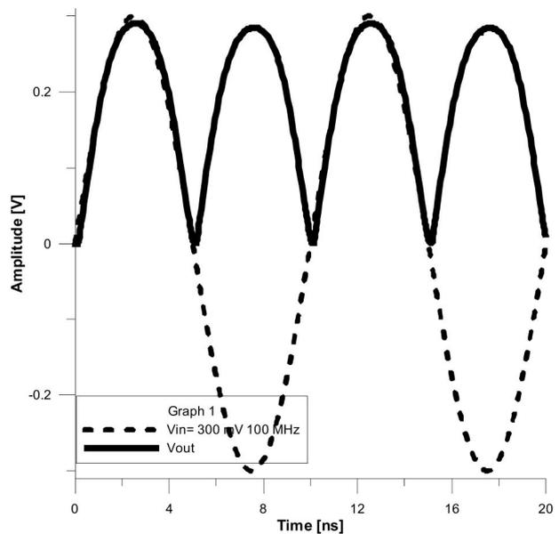
**Figure 8:** Applying the 300 mV sine wave at the input, input and rectified output waveforms of inverting full-wave precision rectifier at a frequency of 100 MHz.
