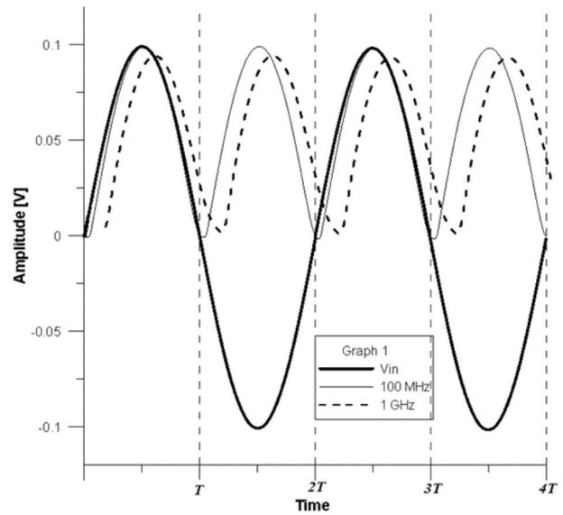
**Figure 7:** Input (sinusoidal) and rectified output waveforms of inverting full-wave precision rectifier of Fig. 4 at 100 MHz and 1 GHz frequencies.
