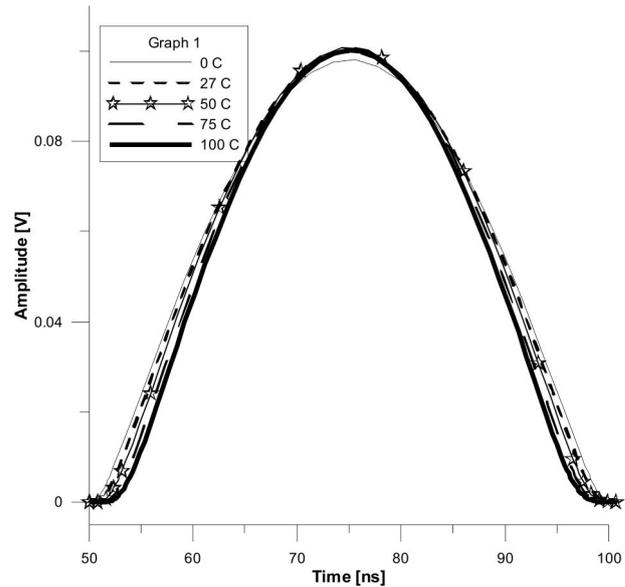
**Figure 12:** The detailed time domain response of the proposed full-wave rectifier of a 100 MHz frequency at different temperatures.
