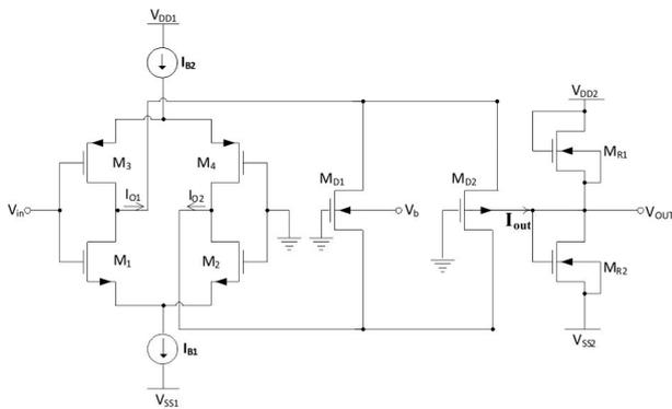
**Figure 4:** Proposed full-wave rectifier circuit.
