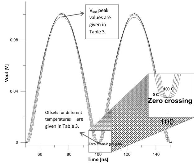
**Figure 11:** Time domain response of the proposed full-wave rectifier of a 100 MHz frequency at different temperatures.
