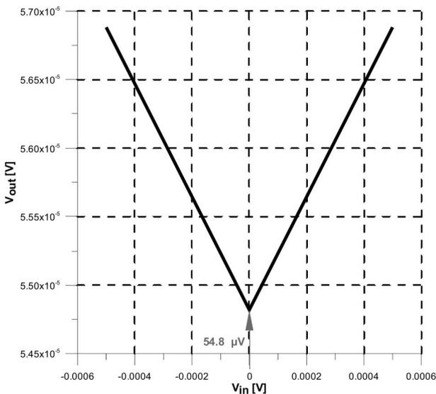
**Figure 6:** Simulated results for DC characteristic at zero crossing regions.
