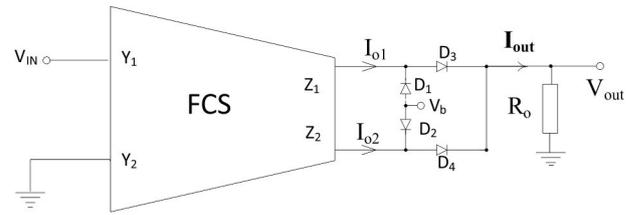
Figure 2: The principle of the proposed rectifier
