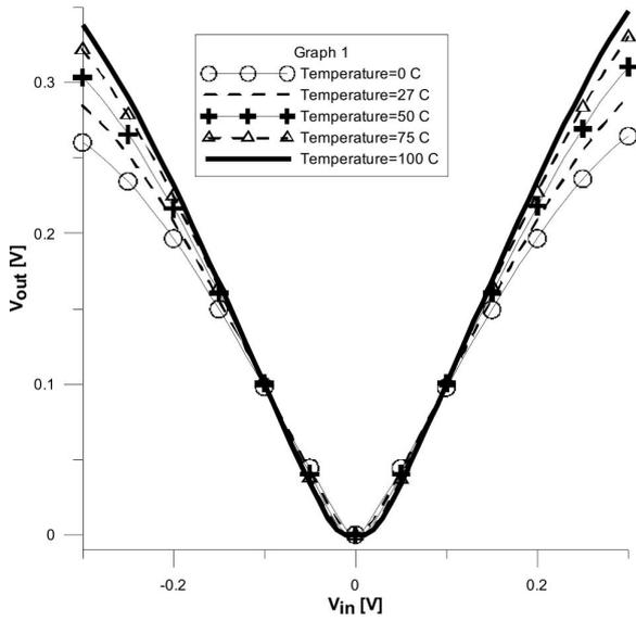
**Figure 9:** DC transfer characteristic of the proposed full-wave rectifier of a 100MHz frequency for different temperatures.
