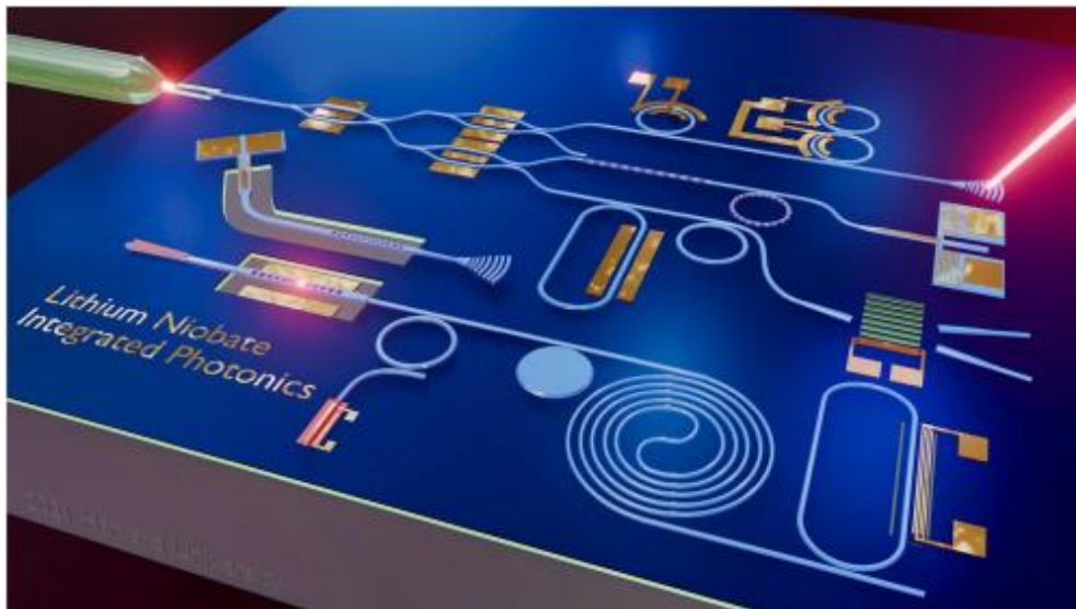
Figure 1: Thin-film lithium niobate has become an established platform for integrated photonics, allowing the integration of many different components on the same photonic chip.
