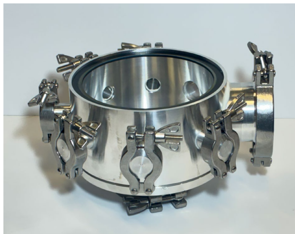
Figure 5: The finished aluminum interface block with mounted KF flanges.
