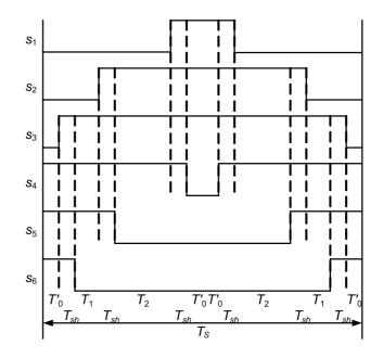
Fig. 6: Modified SVM switching pattern showing the uniform distribution of T<sub>sh</sub>
