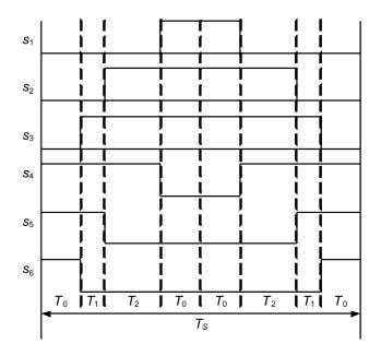
Fig. 2: Symmetrical pulse pattern of SVM for three phase Inverter Bridge
