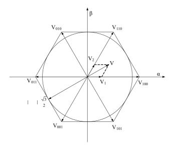
Fig. 1: Space vectors of three phase bridge inverter showing voltage trajectory and voltage vector limit
