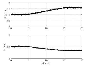
Fig. 10: Ramp up of the speed of IM with VSI  $(U_{DC} = 280 \text{ V})$
