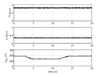
Fig. 13: Motor operation with ZSI when exposed to voltage sag
