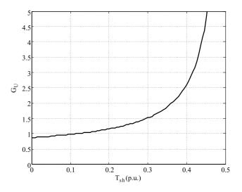
Fig. 8: Maximum voltage gain of ZSI with MSVM
