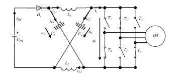
Fig. 3: Z-Source Inverter with induction motor
