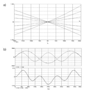
Fig. 7: (a) DC waveform of CDBA and current squarer based current-mode four-quadrant multiplier (b) Transient response of fourquadrant multiplier. Input current signal (top) and together calculated graph and circuit output (bottom) (frequencies of I<sub>x</sub> and I<sub>y</sub> are 3 and 5 MHz, respectively.)
