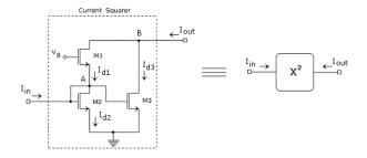
Fig. 4: The current squarer circuit and its symbol
