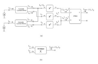
Fig. 2: (a) The building blocks of current-mode multiplier circuit (b) its symbol
