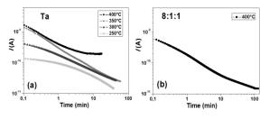
**Figure 3:** *I*–*t* characteristics of the Ta thin films series (a) and the 8:1:1 sample processed at 400 °C (b), measured under the applied voltage of 1V.
